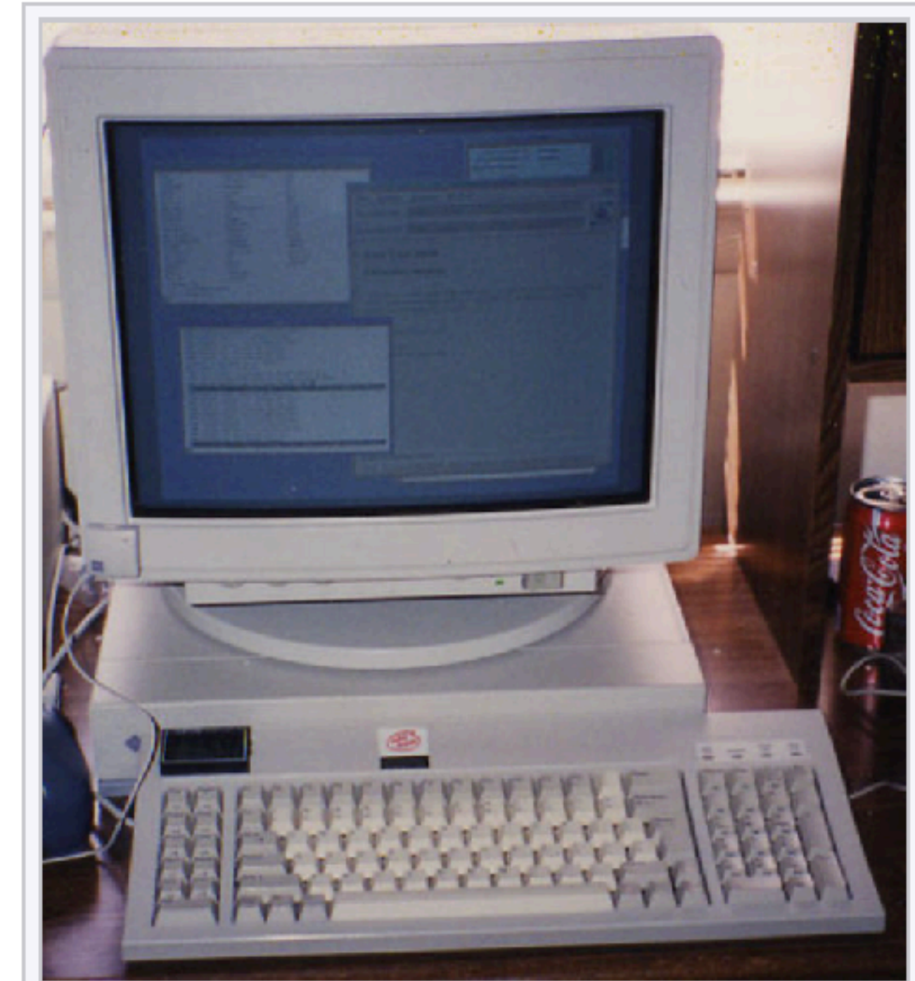
Sun SPARCstation 1+ "pizzabox", 25 MHz SPARC processor, early 1990s
