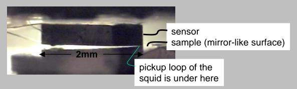
Pickup loop has area ~10um<sup>2</sup>, so a flux of  $1\Phi_0$  corresponds to a field of ~2G.
