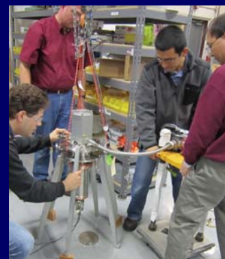
Measuring pulse tube cooler vibrations, at Cryomech, Syracuse
