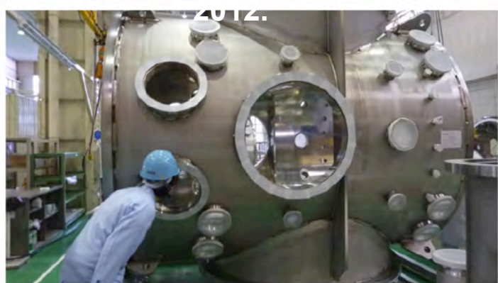
Production of the cryostat.
