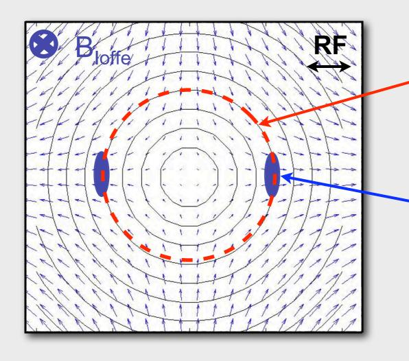
resonance condition forces the trap minimum on a circle
