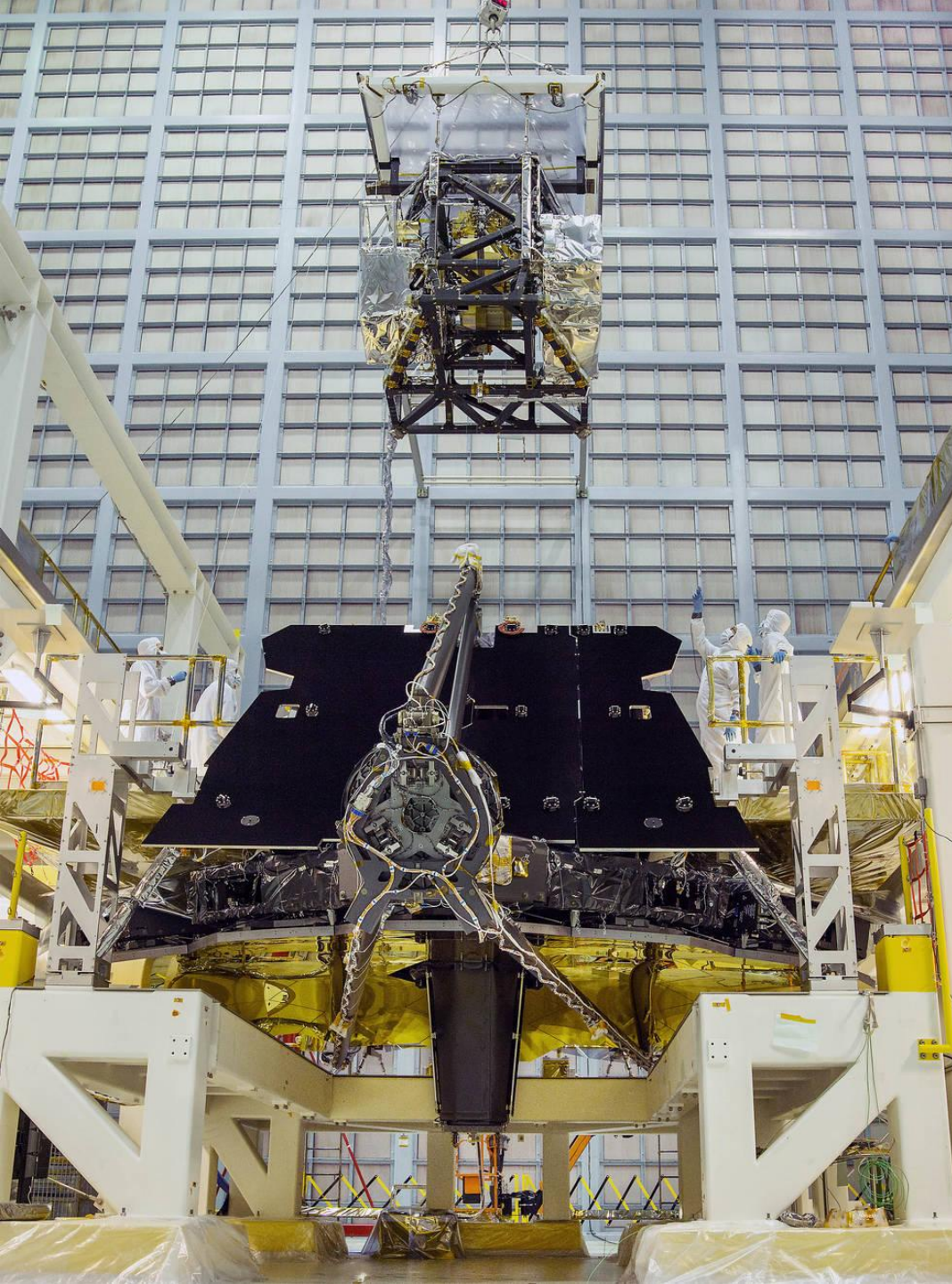
Installed Science Instrument package into Optical Telescope Element (May 2016)
