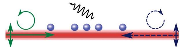
Nanofiber with spin-polarized atoms on one side
