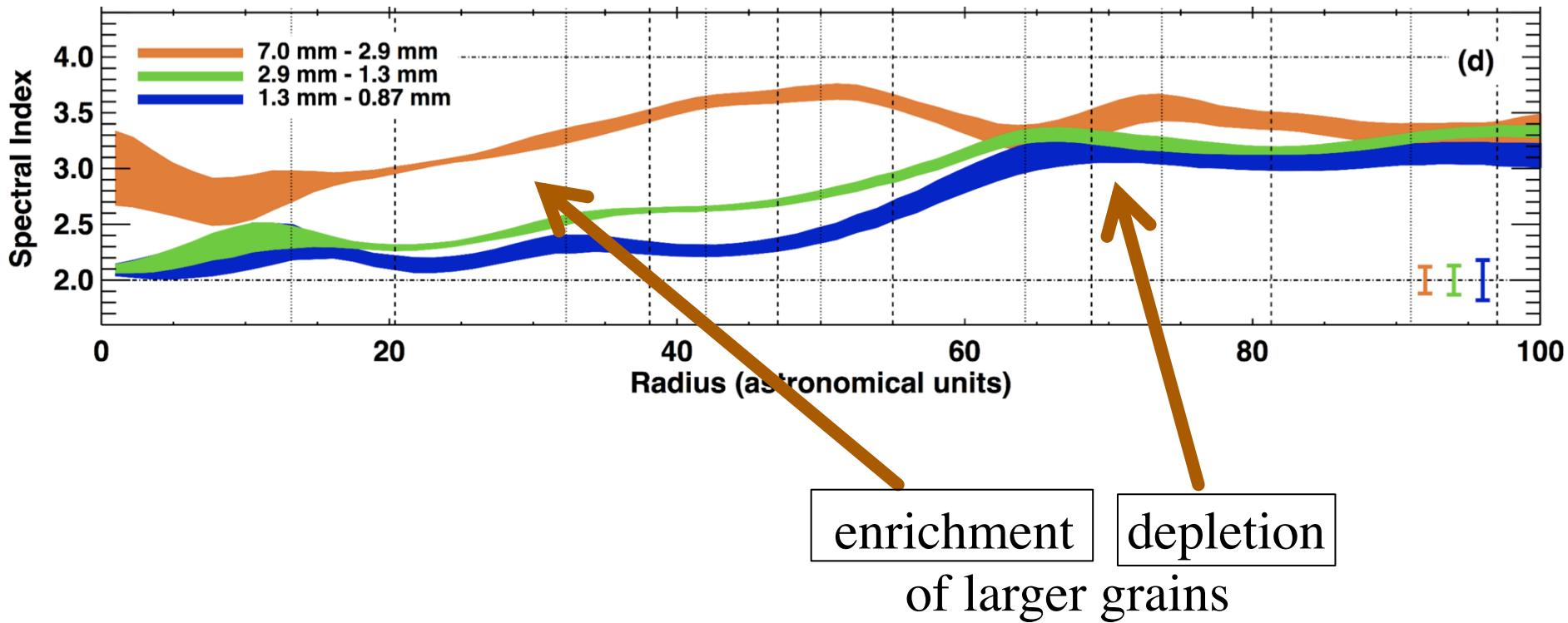
Drop in  $\alpha_{\text{Sp}}$  due to grain size segregation
