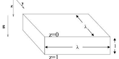
**Initially:** Fully-developed hydrodynamic convection. Density and temperature vary by an order of magnitude across the layer.
