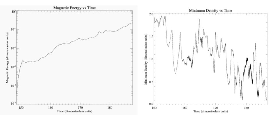
• Magnetic energy vs. time plot suggests that dynamo is still in the kinematic phase. However, the minimum density plot implies that the **localised** magnetic feedback is extremely significant
