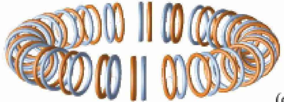
Figure 1. The geometries of the three dynamos considered in this paper: (a) a single pair of Gailitis rings; (b) a small segment of a line of such pairs and some of the magnetic field lines; and (c) an indicative plot of the geometry when the line is bent to form a circle. It is the third of these which, when embedded in a circulating tachocline, can reproduce the observed properties of the solar cycle.
