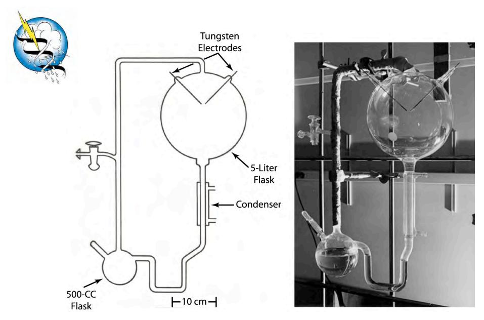
The original Miller/Urey experiment used a reducing gas mixture consisting of methane, ammonia and hydrogen
