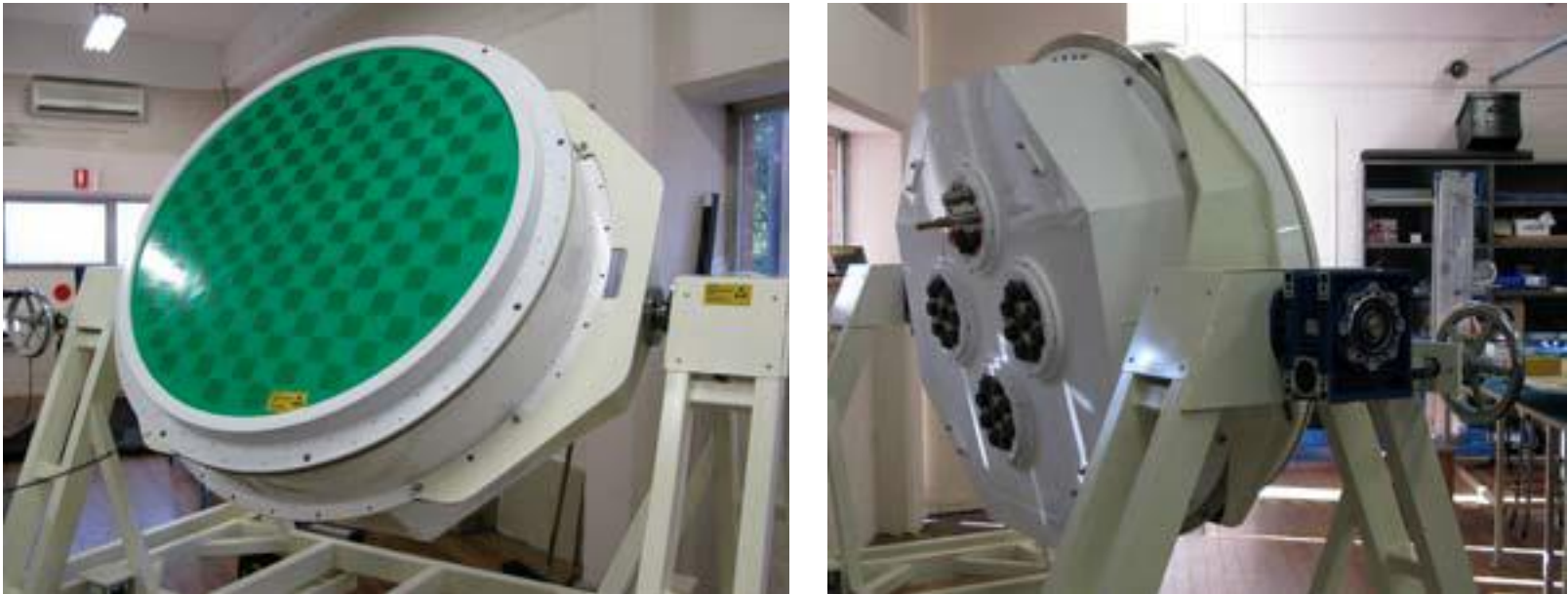
Front view & rear view of the ASKAP PAF
