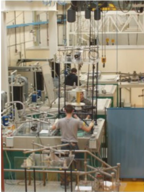
2-forming baths for eROSITA → 8 mandrels/shells simultaneously
