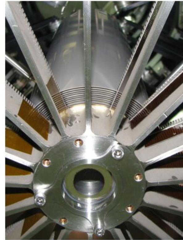
Integration of Shells step by step from inside to outside
