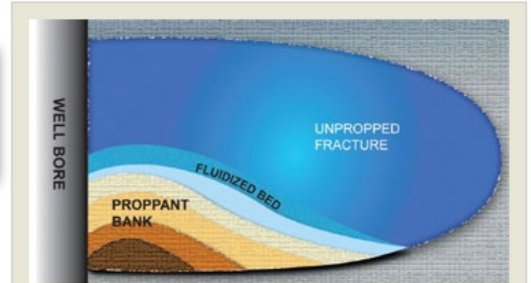
Conventional slickwater bed load proppant transport
