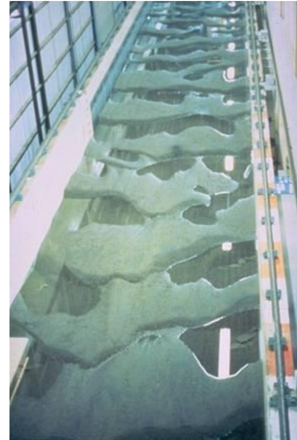
Dunes in a flume in Tsukuba University, Japan: flow turned off. Image courtesy H. Ikeda.
