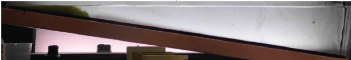
Gravity current along slope at constant speed  $U$
