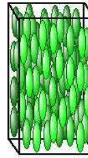
A schematic representation of the nematic phase (left) and a photo of a nematic liquid crystal (above).
