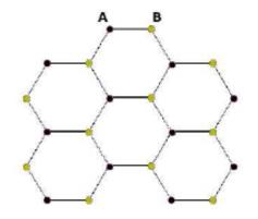
Two triangular sublattices: A and B; one electron per site (half filling)
