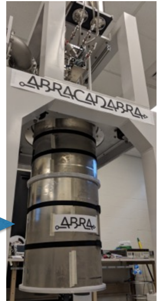
inside dilution fridge ( T = 0.1 \text{ K} )
