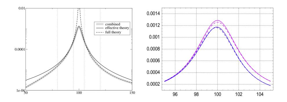
Cross section in  $\text{GeV}^{-2}$  as function of  $\sqrt{s}/\text{GeV}$ , M = 100 GeV. Left: matching off-resonant and resonant cross section Right: LO vs NLO (pole and  $\overline{\text{MS}}$  scheme) Shown is the "partonic" cross section with initial state singularity minimally subtracted.
