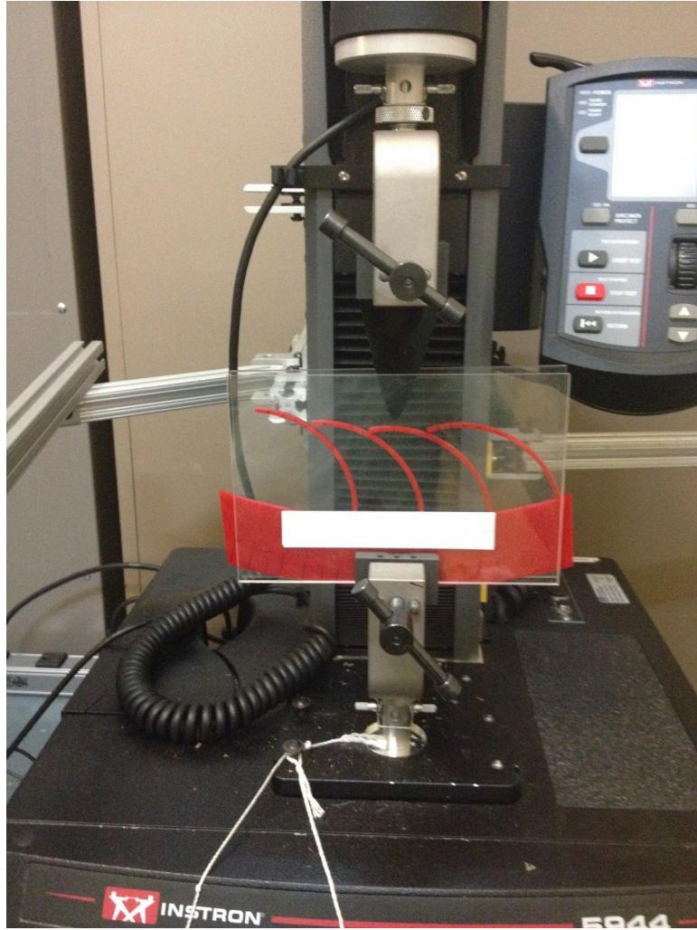
outer boundary is composed of laser-cut leaf springs
