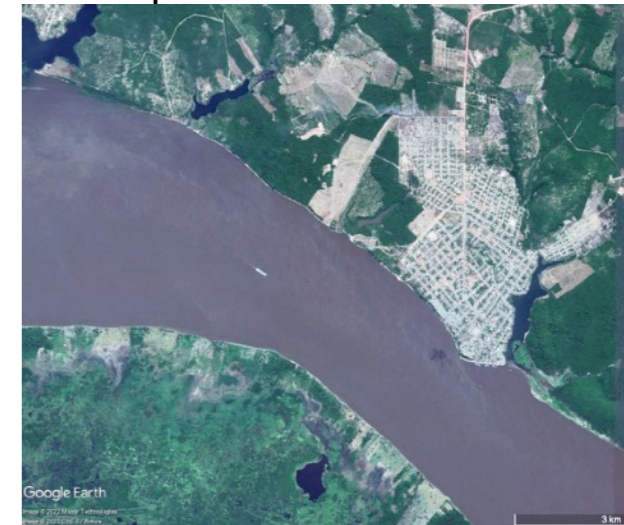
Amazon river, at Obidos width = 2.3 km discharge = 2.2 \cdot 10^5 \text{ m}^3/\text{s} grain size < 100 microns
