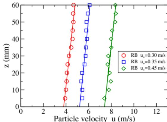
Increasing velocity with increasing flow strength
