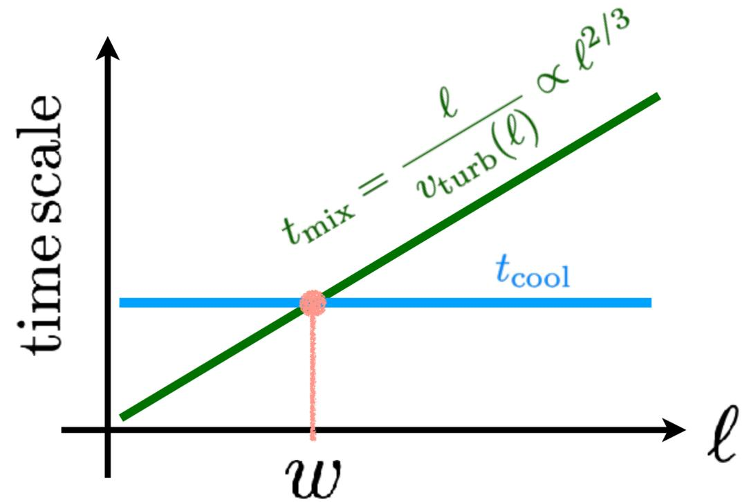
$$\frac{w}{L} = \left( \frac{v_{\text{turb},L} t_{\text{cool}}}{L} \right)^{3/2}$$
