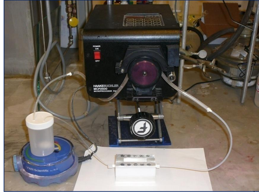
15 mL/min; ~15 psi back pressure, Pulsed intervals: flow and rest
