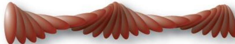
cholesteric: n has helical pitch ( $\sim 1\mu\text{m}$ )
