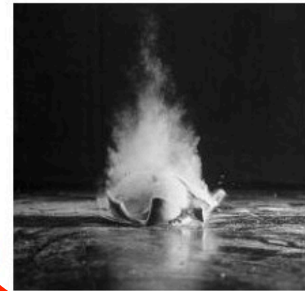
A rubber ball, frozen to near absolute zero by liquid helium, shatters and vaporizes as it strikes the floor. (Source: Getty Images)
