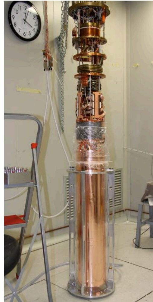
Attached to the Cuoricino dilution refrigerator
