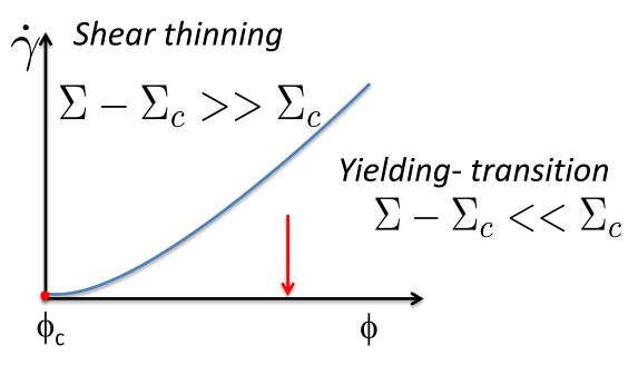
• Line of critical points ending with the jamming transition
