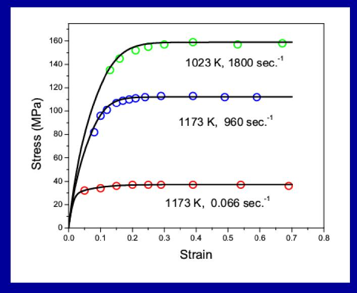
Stress-strain curves for copper at high temperatures, for constant (shear) strain rates as shown. The theoretical curves are from JSL et al.
