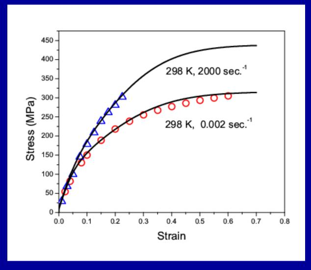
Stress-strain curves for copper at about room temperature, for constant, very different, (shear) strain rates as shown. The theoretical curves are from JSL et al.
