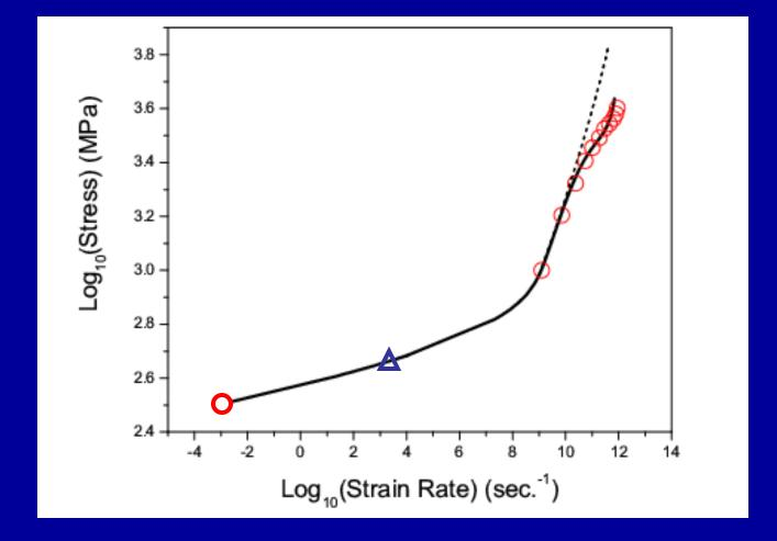
Steady-state stress versus strain rate for Cu at T = 300K. The two points at smaller strain rates are steady-state limits of selected laboratory experiments. The fall-off at the highest strain rates is fit by a heating effect.
