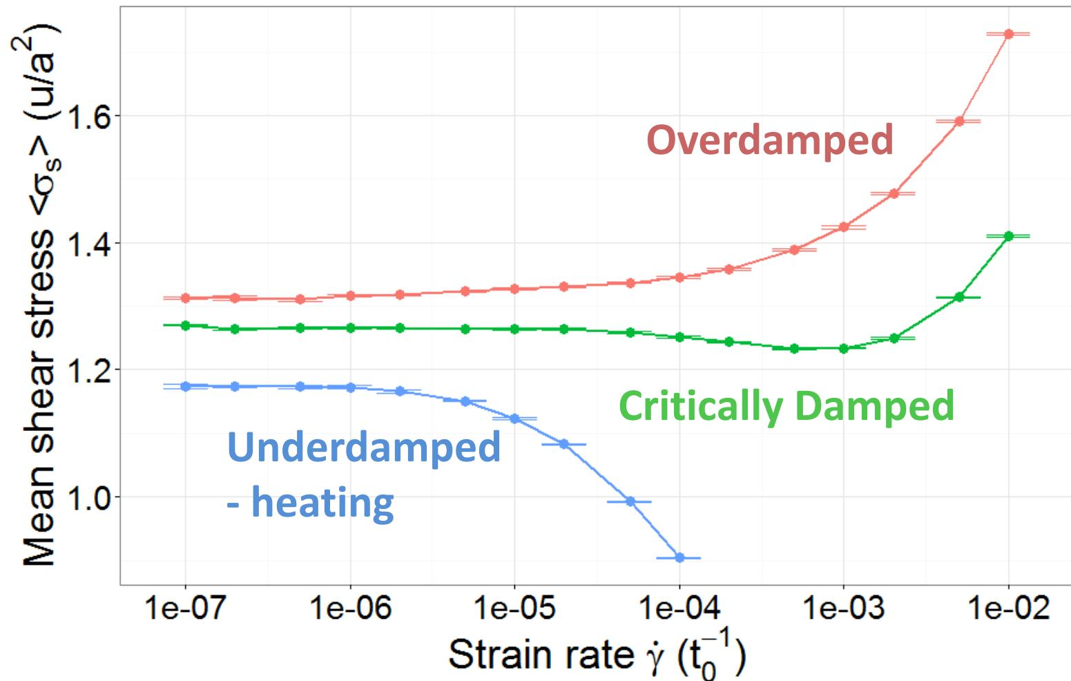
Critical damping takes energy out at same rate generated by plasticity
