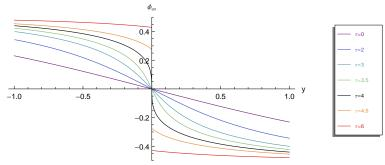
• At finite N the viscous term in Burgers' equation limits the steepness at y = 0:
