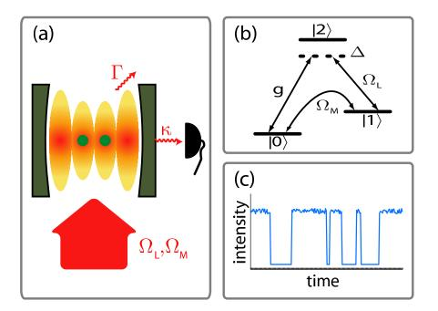
The successful generation of a maximally entangled atom pair is triggered on a macroscopic dark period. The laser should be turned off once the cavity emission stops.
