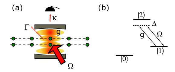
The successful completion of the projection onto the  $\{|01\rangle, |10\rangle\}$  subspace is heralded by the emission of photons as if there is only one emitting atom inside the resonator.
