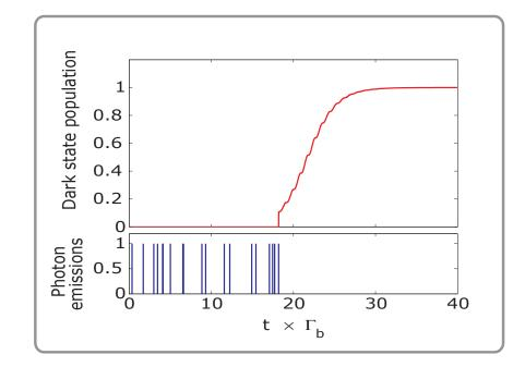
Possible trajectory of the four-level toy model for  $\Omega_{\rm b} = \Gamma_{\rm b}$  and  $\Gamma_{\rm d} = 10^{-2} \Gamma_{\rm b}$ . The upper figure shows the population in the dark state  $|b\rangle$ ; the vertical lines mark photon emissions. The population in  $|b\rangle$  eventually reaches one.
