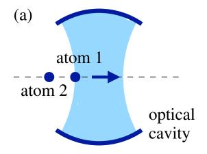
Two two-level atoms can be prepared in a maximally entangled state by moving them slowly into an optical cavity.
