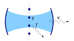
g: atom-cavity coupling constant $<math display="block">\kappa: spontaneous cavity decay rate$  $<math display="block">\Gamma: spontaneous atom decay rate$
