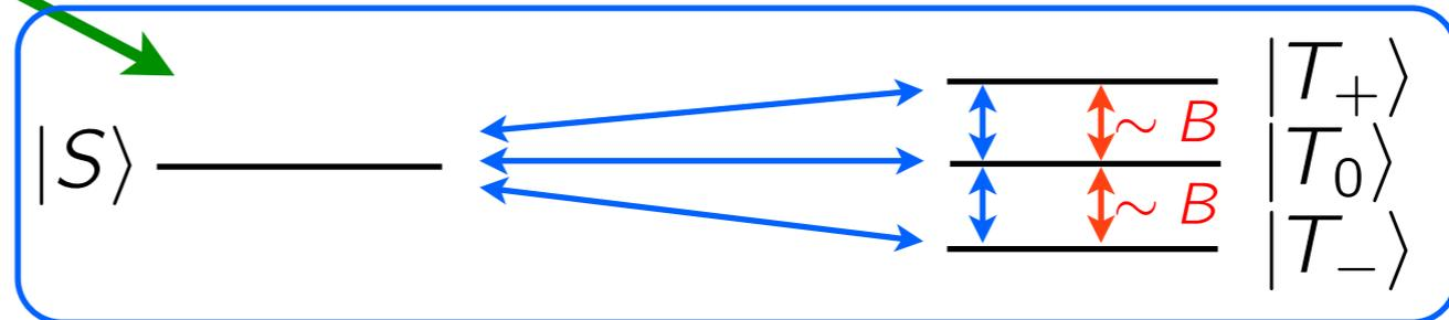
Decoherence due to local nuclear spin baths breaks symmetry and enables the magnetometer.
