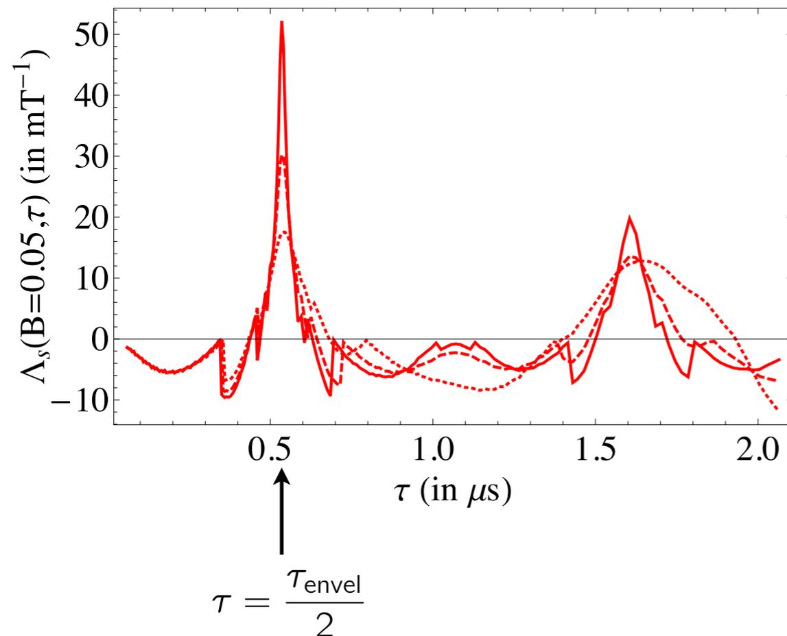
Scanning over different laser-timings reveals resonances of increased sensitivity.
