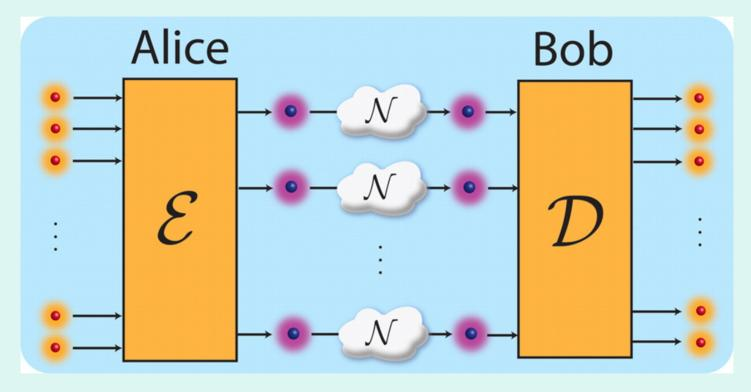
$$Q(\mathcal{N}) = \max\left(\frac{\# \text{ quantum bits sent}}{\# \text{ channel uses}}\right)$$
