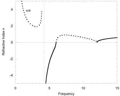
Index of refraction vs Frequency (GHz)
