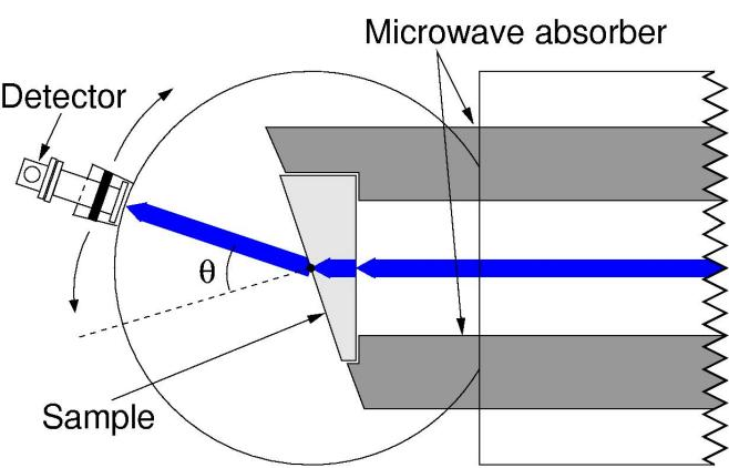
A schematic diagram of a microwave scattering setup. A blue horizontal beam passes through a sample (represented by a grey rectangular block) at an angle  $\theta$  relative to the normal. The beam is detected by a detector positioned at an angle  $\phi$  from the vertical axis. A microwave absorber is located behind the sample.
