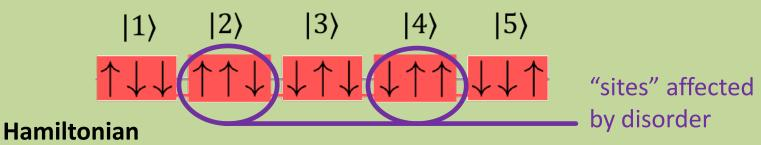
$$H_{\rm A} = \frac{\Omega}{2} \sum_{b=1}^{2L-2} \left[ \left| b \right\rangle \left\langle b+1 \right| + \left| b+1 \right\rangle \left\langle b \right| + h_b \left| b \right\rangle \left\langle b \right| \right] \quad \text{with} \quad h_b = \frac{\delta V_{b/2}}{\Omega} \left[ 1 + (-1)^b \right] \\ \text{site dependent disorder}$$
