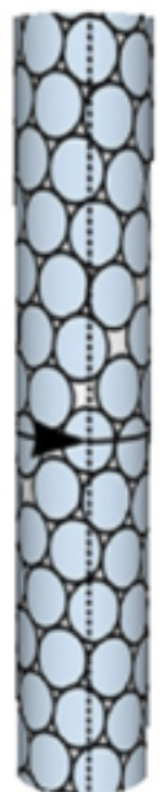
Helical "line-slip" defects in a triangular lattice
