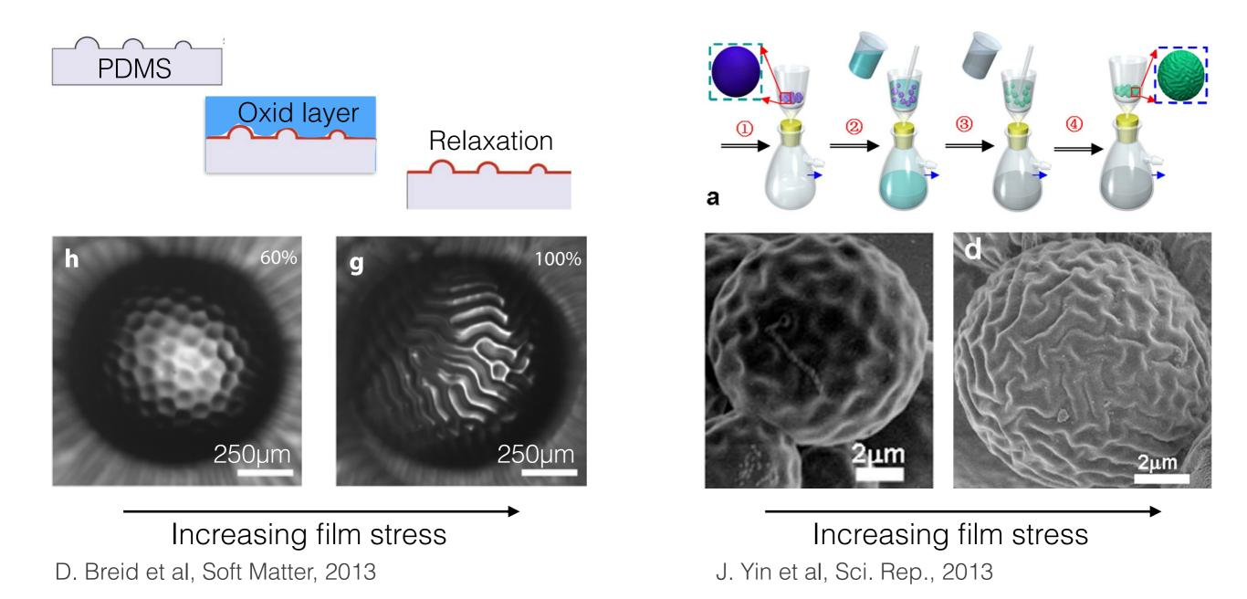
Experiments suggest: Curvature and film stress determine wrinkling patterns
