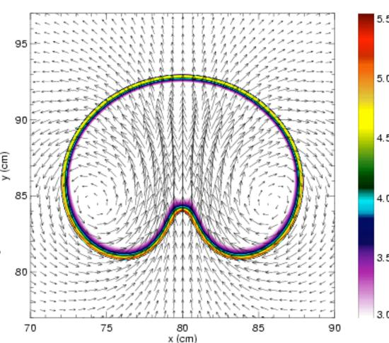
Simple semianalytic model for this case: flame speed ~ rise speed between 30-50 flame thicknesses in size
