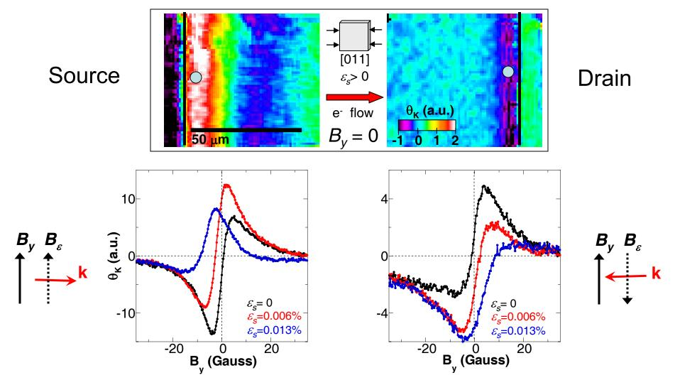
• At opposite ends of the channel, the Hanle curves shift in *opposite* directions with increasing strain. *The (diffusive) spin current at the drain is flowing against the charge current*. See also M. Hruska *et al.*, Phys. Rev. B **73**, 075306 (2006).
