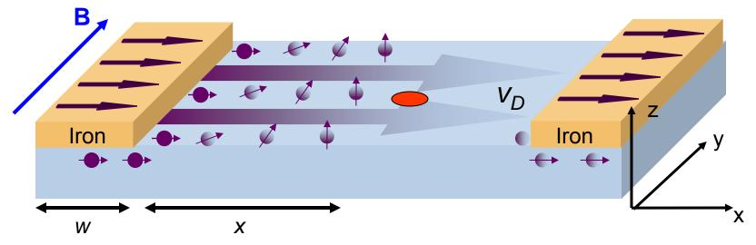
D = diffusion constant  $v_d = \mu E =$  drift velocity  $\tau_s =$  spin lifetime
