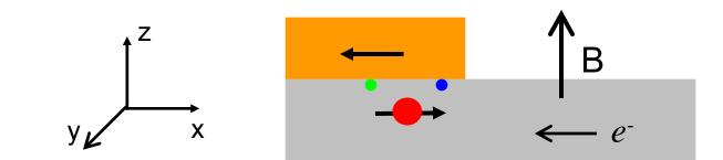
$$S_{x}(B) = \int_{0}^{L_{eff}} dx_{1} \int_{0}^{L_{eff}} dx_{2} \int_{0}^{\infty} dt \frac{S_{0}}{\sqrt{4\pi Dt}} e^{-\frac{(x_{2}-x_{1}+v_{d}t)^{2}}{4Dt} - \frac{t}{\tau_{s}}} \cos(\frac{g\mu_{B}B}{\hbar}t)$$
