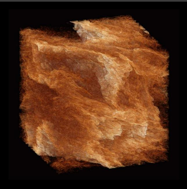
A snapshot of  $\nabla \times \boldsymbol{u}$  at Mach 6, grid resolution  $1024^3$  [Kritsuk et al. 2007]
