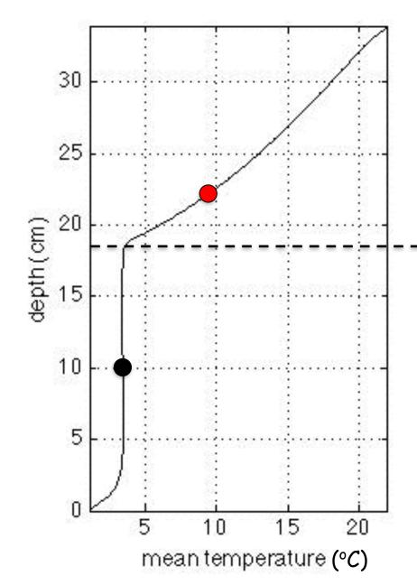
Stratified zone = heat transfer by conduction
