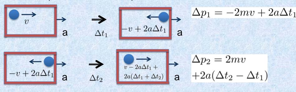
$$F = \frac{\Delta p_1 + \Delta p_2}{\Delta t_1 + \Delta t_2} = \frac{2ma\Delta t_2}{\Delta t_1 + \Delta t_2} \approx ma$$
