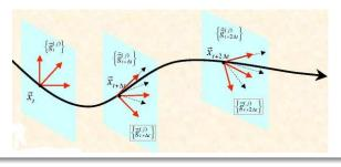
Jacobian matrix : orthogonal frame  $\to$  non-orthogonal frame  $\to$  QR decomposed into an R-matrix + Gram-Schmidt frame  $\to$  next Jacobian matrix, and so on
