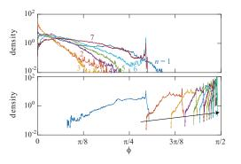
histogram of angles between  $S_n$  (n leading Floquet vectors) and  $\bar{S}_n$  (the rest), accumulated over the 400 orbits :
