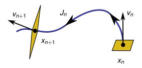
$$x_{n+1} + z_{n+1} = f(x_n) + J_n z_n, \quad J_{ij} = \partial f_i / \partial x_j$$
